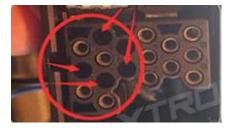
Please remove the plastic frame as shown before installing the head units.
